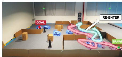
Figure 6: A representative failure case under limited depth FoV. The red trajectory represents the robot initially navigating out of the dead end. The blue trajectory indicates it re-entering the same trap after missing a traversable opening, before eventually recovering and reaching the goal.
